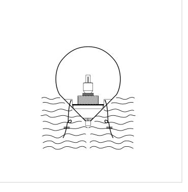
Lights that are installed at the edge of a pool must be operated with a voltage of 12 volts due to legal requirements. That's why we also offer our MAG model in a low voltage version.
